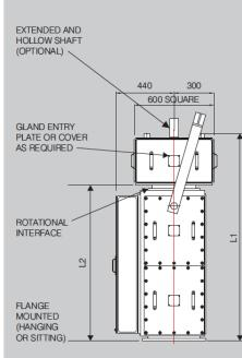
Dimensions L1 & L2 are variable and to be advised when number, size and voltage requirements of slip rings are known
