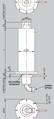
Dimension L is determined by the size and number of rings and is detailed on our quotation
