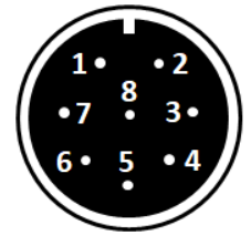
M12/8 Pin female socket (front view of the cable-mounted socket)
